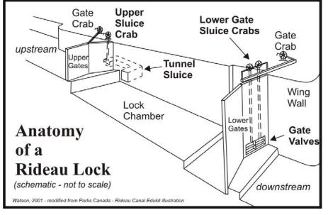
upstream water level. Note that the sluice valves are opened slowly to prevent excessive turbulence in the lock. As the water depth in the lock chamber increases, the lock staff fully open the valves.
